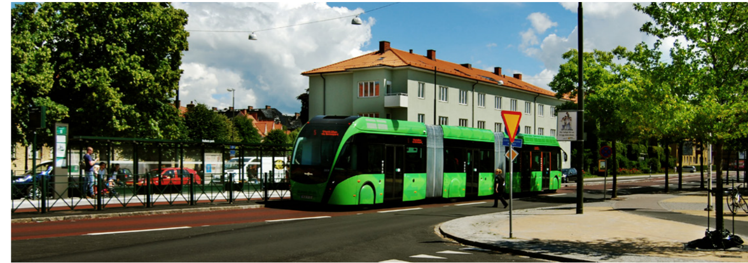
MalmöExpressen – a new, 24 m long, double articulated bus, powered by a hybrid engine (gas and electricity), developed for the City of Malmö together with the regional public transport authority (Skånetrafiken), Nobina and Van Hool (Photo: Åsa Svensson).
